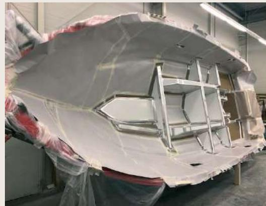
Our German Lloyd ISO certified Shipyard, with its ultra-modern, air-conditioned manufacturing facility gives us the setting and the ability to fabricate a superior laminated boat hull. The combination of Isophthalic acid resin, powder-bounded chopped mats and adapted woven fiberglass offer a high tensile strength shell for our fast planing hulls.
